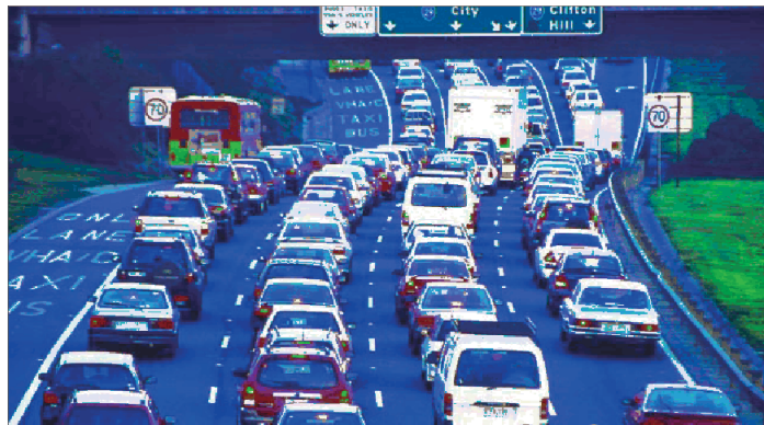
Example of road space reallocation showing a dedicated bus and taxi lane in Melbourne, Australia.
