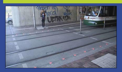
Flashing lights on ground (LED on gauge limit)
