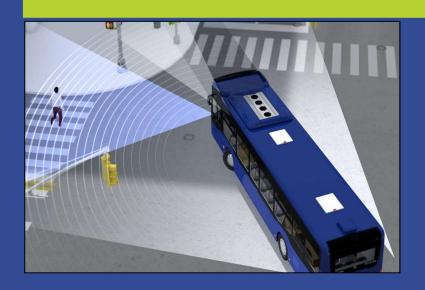
Pedestrian (and cyclist) blind spot detection (MobilEye Shield Plus)
