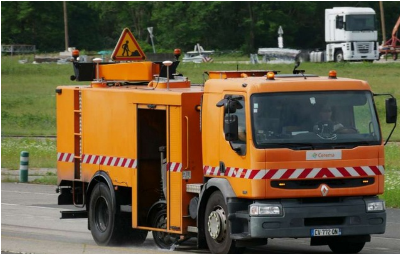
SCRIM (Sideways- force Coefficient Routine Investigation Machine)
