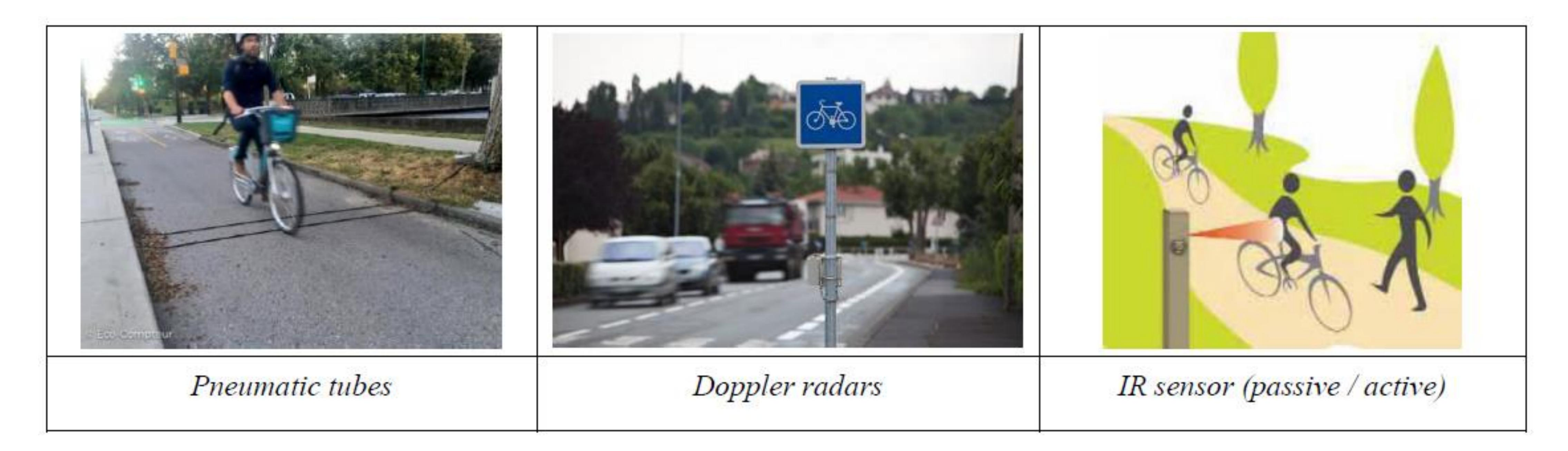
Non-intrusive sensors for temporary counting on sites with mixed traffic (soft/motorized modes)
