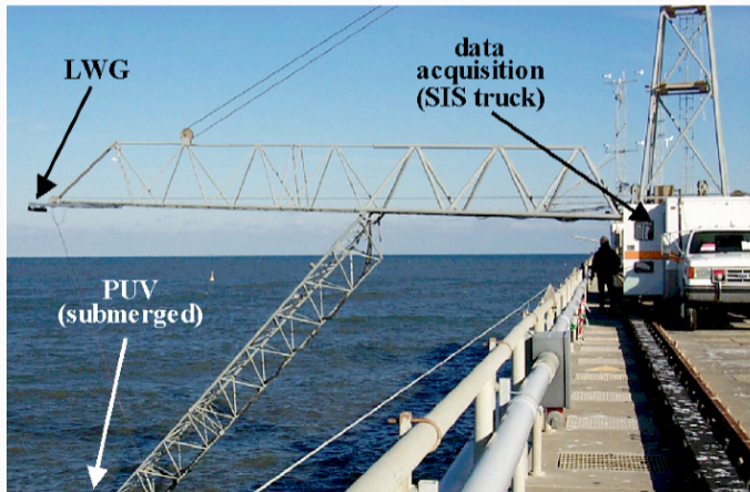
Deployment over the Field Research Facility pier at Duck, NC
