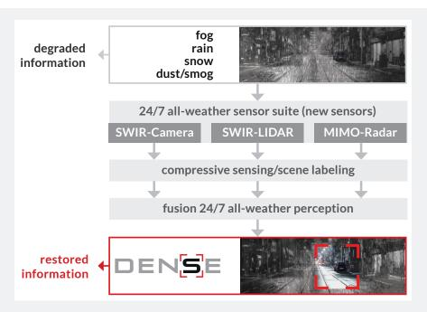
➤ The DENSE 24/7 all-weather sensor suite combines Radar, a Short Wave Infrared (SWIR) gated camera sensor and LIDAR. In addition, a mobile Road State Sensor assesses the road surface conditions.
