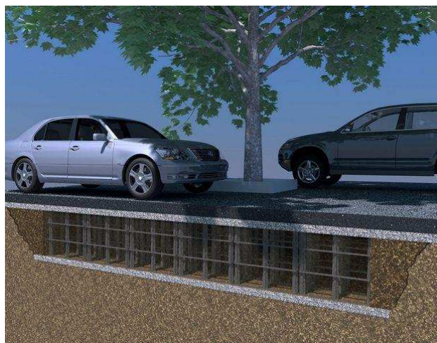
Figure 34 : Cellule Silva cell - Grenmax (droite) - Deeproot, 2017 (gauche)
